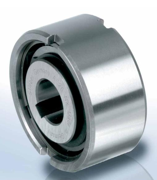
ype AE is a roller type freewheel non-bearing supported. Bearings are required to support axial and radial loads. Lubrication and sealing must also be provided by the installation. Nominal outside diameter is a standard ball bearing dimension.
